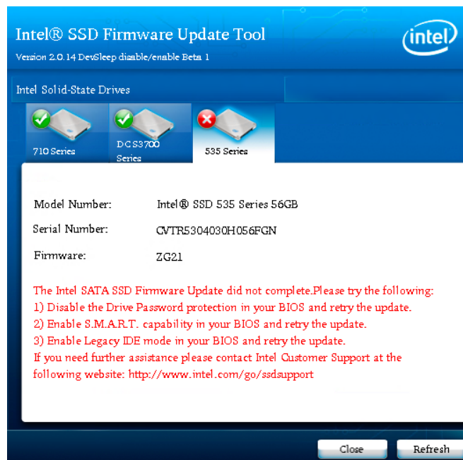
Figure 10. Firmware Update Failure Message
